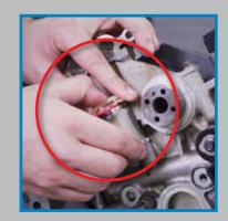
B. Once the tensioner is installed, remove the clip. This step does not activate the tensioner. The clip is simply used to avoid accidental activation while installing.
