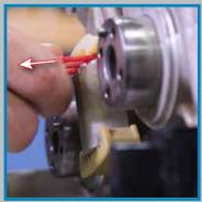
C. After the cam phasers and chains are installed, you must then activate the tensioners. Press on the chain above the tensioner pad allowing the tensioner plunger to fully compress and release. Make sure the tensioners properly activate and apply spring pressure to the chains.
