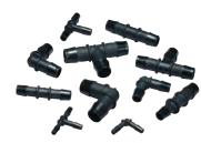
These Dayco glass-filled nylon, straight, "Y", elbow, tee and reducing connectors produce a leak-proof splice between vacuum line tubing, fuel line hose, coolant hose, or other small I.D. hoses and are ideally suited for all jobs requiring 3/32", 1/8", 5/32" and 3/16" I.D. connections. A molded circumferential flange provides a hose stop that assures that the hose is inserted to the proper depth. The connectors are packaged and sold in poly bags, one per package.
