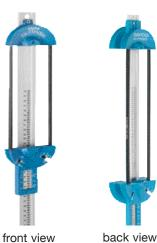
Measures all multi-ribbed belts (competitive or OEM) up 115" in effective length and indicates the corresponding Dayco replacement belt size. The Dayco Factfinder® Gauge III measures V-Belts up to 28/32" top width and 100" effective length.
