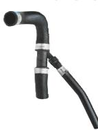
The Dayco Branched Radiator Hose is an ideal aftermarket replacement for OEM branched hose. The hose's all EPDM construction resists the effects of oil, mud, salt and ozone, while its knitted rayon reinforced inner tube offers resistance to temperature ranges of -40°F (-40°C) to +257°F (+125°C). Leak proof junctions ensure long service life and unrestricted flow. This hose meets SAE J20R4, Class D-1, Type EC electrochemical requirements as specified in SAE J1684.
