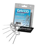
The Dayco Tensioner Retainer Pin Set is designed for the installation and maintenance of timing belt tensioners. To safely retain the hydraulic pin of a timing belt tensioner in a compressed state during servicing, Dayco recommends the use of this handy Tensioner Retainer Pin Set. Consisting of six different sized spring hardened steel pins, the set accommodates a wide variety of timing belt tensioners, including certain serpentine belt applications.
