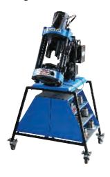
This stand will give you the safety of a secure stand with versatility of casters to allow you to safely and easily move your crimper set up anywhere at your location. Dayco's D206 crimper can be easily mounted on top of this stand using four attachment bolts. With the available bottom shelf, this stand is ideal for utilizing Dayco's Die Storage Cabinets to create an easy access hydraulic set up that is convenient and practical.
