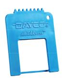
By simply placing the notched area lengthwise over the ribbed section of the belt, this pocket size device quickly and easily identifies the potential of serpentine belt failure. If there are more than four cracks per inch in the belt, trade practice recommends the belt be replaced.
